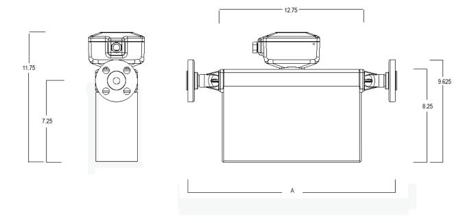
Shown with 1/2", 300# flanges and NexGen SFT200 Mass Flow Transmitter
