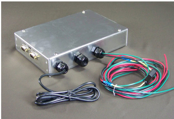
Figure 4-25. Junction Box Cables - Printer on Left, Truck Power on Right
