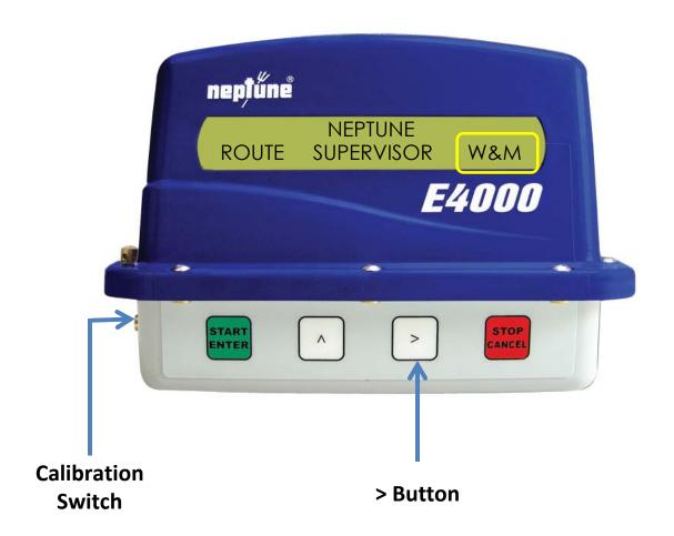
Starting from the root menu, remove the seal screw from the left side of the register and depress the internal calibration switch using a paper clip or small Allen key (3/32" is ideal).
