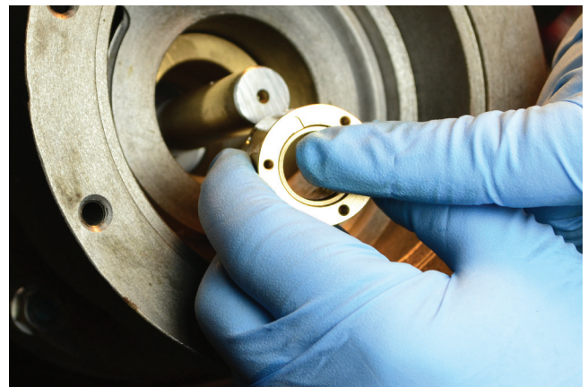
28. Install the new seal into the housing. Align the notch in the seal sleeve with the hole in the shaft.
