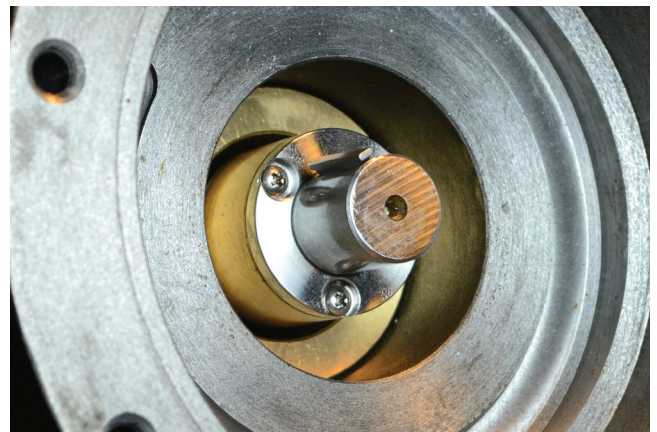
34. Shaft key properly installed. If you are replacing the impeller only and have not removed the key, verify that it is still seated correctly and the key and shaft are free of burrs and foreign material.
