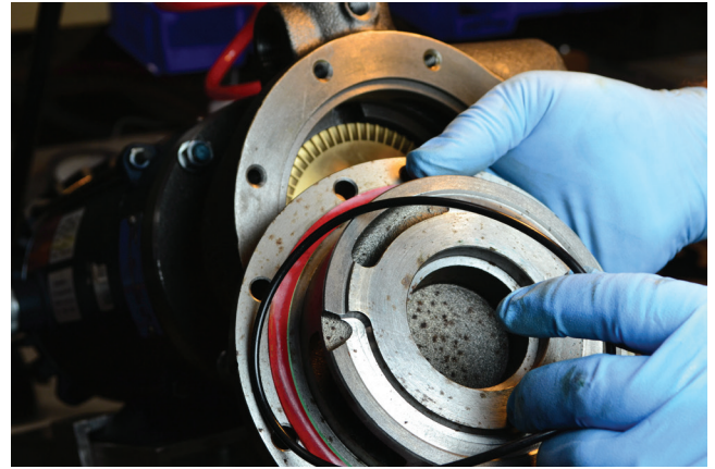
36. Remove the old cover o-ring. Make sure the cover surface is clean and install the new o-ring. If cover shims were used, put them back in place if they were removed during disassembly.
