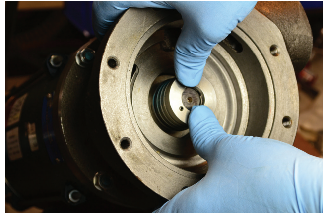
12. If you have difficulty seating the housing, the old housing can be used to press it in place.
