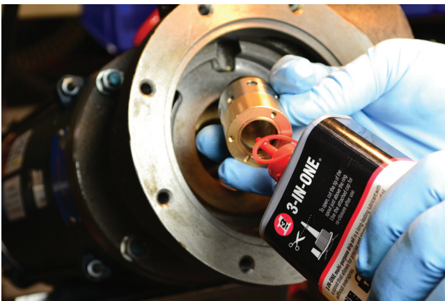
27. Apply oil to the o-ring on the other end of the seal sleeve.
