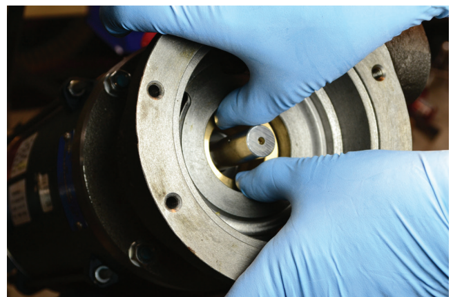
22. Install the new seal housing and press it in until fully seated.
