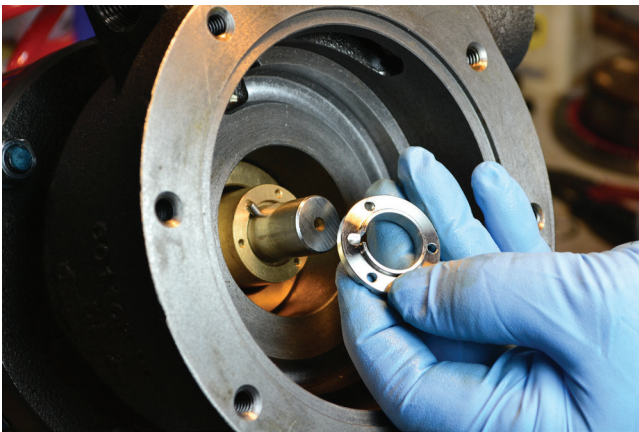
31. Install the seal clamp ring that was previously removed from the new seal cartridge. Align the notch in the ring with the drive pin.
