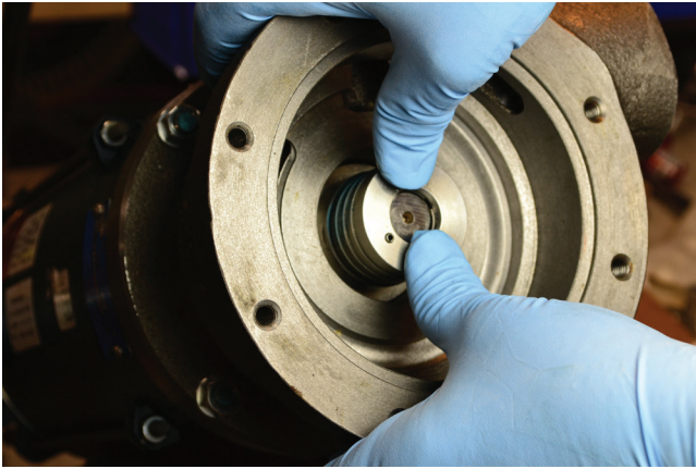
23. If you have difficulty seating the housing, the old housing can be used to press it in place.
