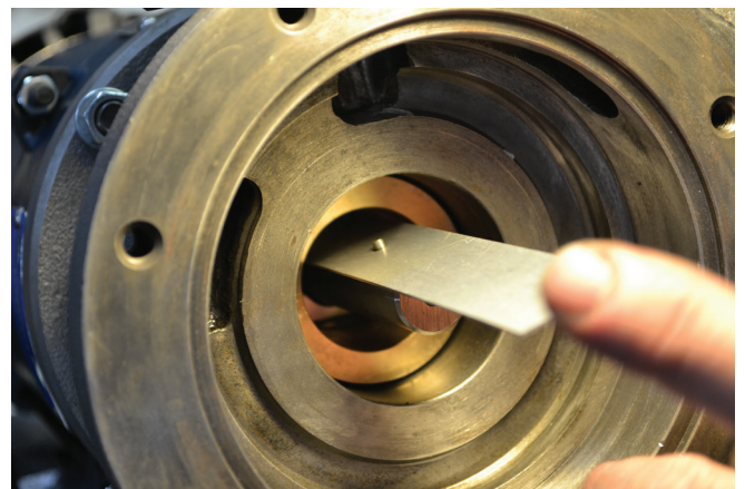
16. Correctly shimmed seal housing. At this point, remove the pin, shims, and seal housing before continuing.
