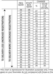
gears on your flowmeter do not correspond with those on the chart, contact your nearest RSM authorized distributor, giving flowmeter size, register type, dial capacity and unit measure.
