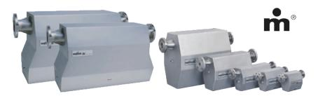
Red Seal Measurement offers a broad range of Coriolis mass meters with flow rates ranging from 0.09 kg/min (0.20 lbs/min) on the 1/8" M012 model to 6,804 kgs/min (15,000 lbs/min) on the 4" M400 model. All models are available with different flange sizes and pressure ratings to meet all application requirements.
